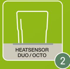
Place the microwell on the heating block
